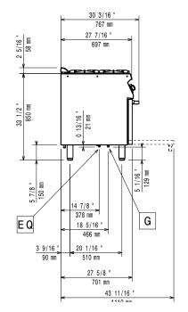
EQ = Equipotential screwG = Gas connection
