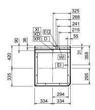
CWI = Cold Water inlet XD = Detergent connection
