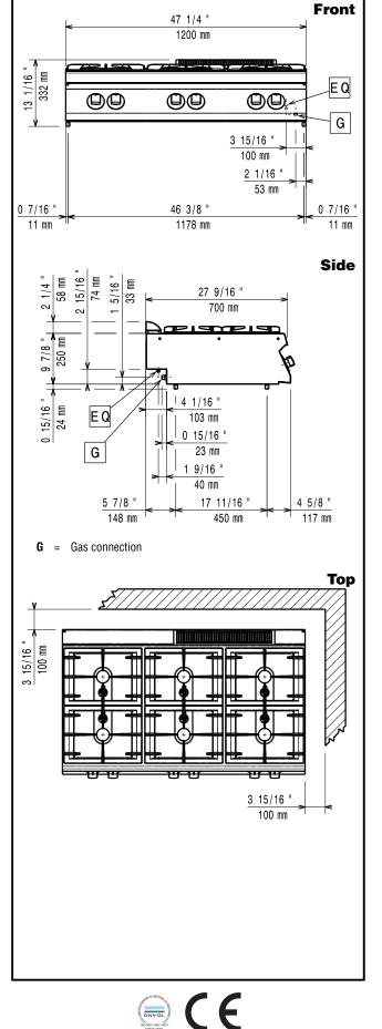
Modular Cooking Range Line EVO700 6-Burner Gas Boiling Top
